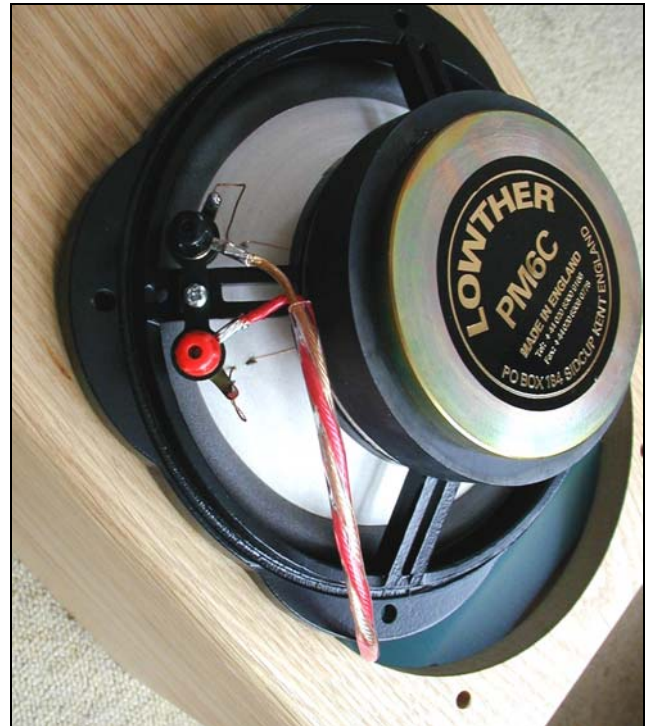
Driver, ready for installation
